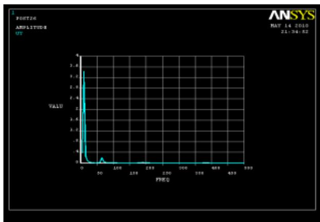
*Fig.3 : Variation of displacement with frequency for Carbon Reinforced Composites for 0° orientation.*
