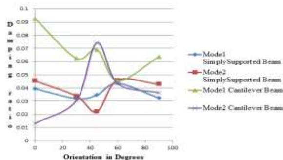
Fig.8 variation of damping ratio with fiber orientation for Carbon Reinforced Composites
