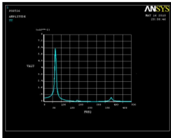
Fig.6 : Variation of displacement with frequency for 0<sup>0</sup> orientation of simply supported beam.
